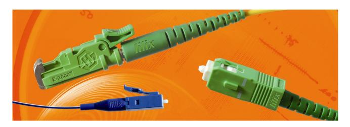
The connector integrated lilix FTTx Reflector 1625/1650 nm selectively reflects in the wavelength range of either 1625-1675 nm or 1645-1675 nm. With its low insertion loss and high reflectance it is the ideal optical termination for link monitoring of FTTx networks via Central Office based measurements at 1625 or 1650 nm, e.g. with modern OTDR. Since the operating channels remain undisturbed, link monitoring may be executed at any time.
