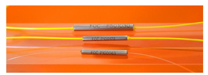
The lilix FTTx Reflector 1625/1650 nm selectively reflects in the wavelength range of 1625-1675 nm or at 1645-1675 nm. With its low insertion loss and high reflectance it is the ideal optical termination for link monitoring of FTTx networks via OTDR (optical time domain reflectometer) measurements at 1625 nm or 1650 nm from Central Office. Link monitoring is possible at any time since the operating channel remains undisturbed.
