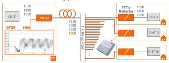
The picture shows a 1x64 PON in which every splitter branch is terminated with an FTTx reflector, such representing the subscribers. The optical line length is 10 km in total (including launch fiber). Every reflector can be clearly identified in the OTDR trace and may be
